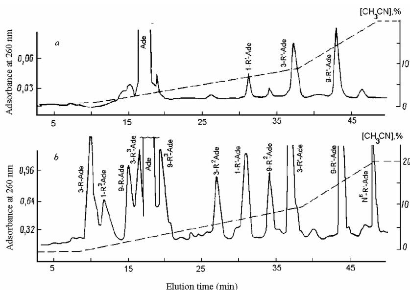
Fig. 3. HPLC on the column (4x150 mm) Bio-Sil ODS-5S for the mixture of adenines alkylation by thiotepa during a day in neutral conditions at room temperature and in adenine-thiotepa- $\text{HClO}_4$  3:15:0.1 ratio (a) and after 8 h of heating at 100 °C and in adenine-thiotepa 1:2 ratio (b). 1, 3, and 9 — sites of adenine alkylation. The structures of R, R<sup>1</sup>, R<sup>2</sup> and R<sup>3</sup> radicals are presented in scheme 3.
