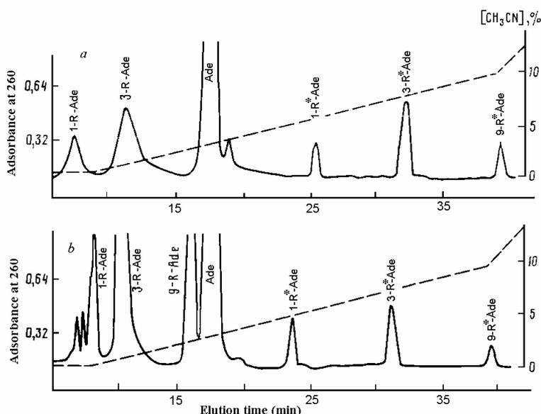
Fig. 2. HPLC on the column (4x150 mm) Bio-Sil ODS-5S for mixture of adenines alkylated by monoaziridinediethylphosphate at 37 °C during a day and in adenine-MAEP- $HClO_4$  1:1:0.1 ratio (a), the same mixture after acid (0.5 N HCl, 100 °C, 1 h) hydrolysis (b).  $R$  — radical with amide bond cleavage,  $R^*$  — radical without such cleavage.
