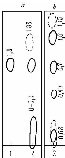
Fig. 4. Separation in the system *i*-propanol — ammonia (25 %) — water 7:1:2 ratio of adenine products alkylated by thiotepa (37 °C, 24 h) on the paper Filtrak FN-12 (a) and plates Silufol UV-254 (b): 1 — adenine, 2 — reaction mixture. Numerals near the spots — their  $R_f$  comparative to adenine. Starting pH — 7 (a) and 4.5 (b). Operating conditions for experiment are presented in section «Materials and methods».
